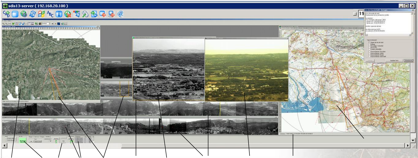
Areal Photo - System Status - Alerts - Sector live sequence - b/ w image - Panorama view - color live seq. - Coordinates (WGS,LL,DCFI)- Digital Map
