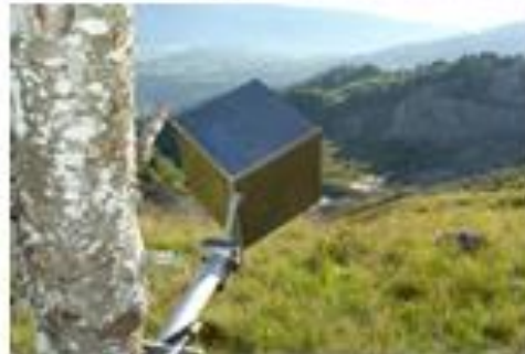
Radar reflectors used for high precision tracking of displacements (e.g. in forested areas)
